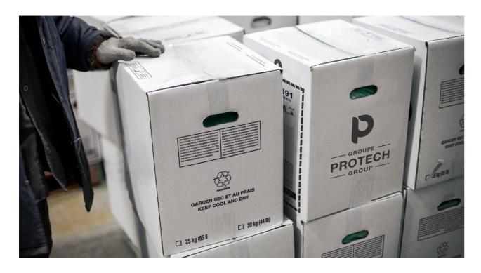
Thermoplastic coatings can be formulated differently. Poor storage conditions will affect them in different ways despite having the same storage and condition period. Variations in storage temperatures may lead to a reaction within the container that will ultimately make the thermoplastic difficult to apply.
